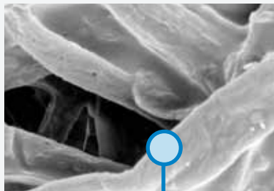
10 Micron Cellulose Media (600x)
